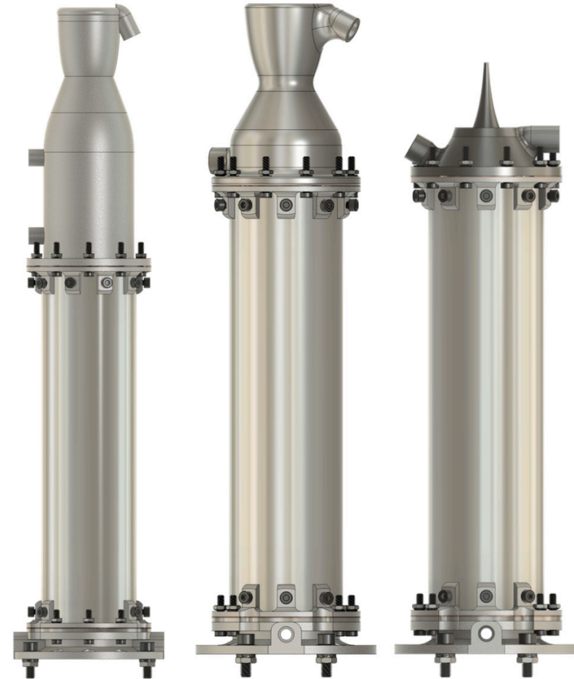
DESIGN VARIATIONS OF ICARUS (V1, V2, 1KN AEROSPIKE)
