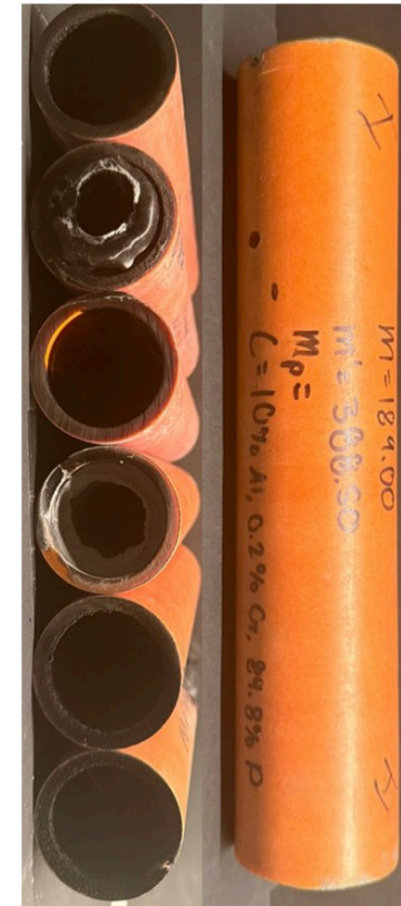
Post-fire, fuel grains (L)
